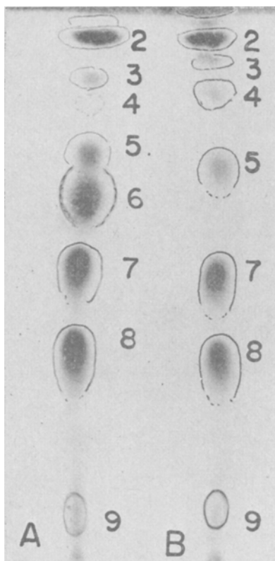
FIG. 1. Thin-layer chromatograms of steroids in aerated cholesterol sol. A , No alkaline treatment. B , Hot alkaline treatment.
