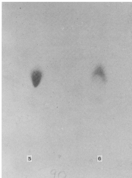
FIG. 3. TLC of phosphatidyl(dioleoyl)hydroxy-L-proline eluate from silicic acid column. Channel 5—pure phosphatidylhydroxy-L-proline; Channel 6—lecithin and lysolecithin from egg (The stain employed was that of Long et al. for phosphorus compounds (17).).
